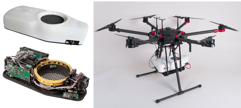
Figure 3. Photograph of the CH 4 laser spectrometer with and without the protecting cover (left). The main building blocks are the TO3-packaged QCL installed on a three-axis stage with additional TEC stabilized heatsink, the SC-MPC with 10 m effective path length, the MCT detector, also with TEC stabilized heatsink, and five PCBs incorporating the hardware electronics: an icw laser driver, a DAQ unit with extension board, a power-supply module, the OEM TEC-board of the detector, and a custom TEC-board for laser and detector heatsinks. The heatsinks of the laser and detector are, in addition, actively air cooled with fans. Picture of the CH 4 sensor installed on the hexacopter (Matrice 600, DJI).
