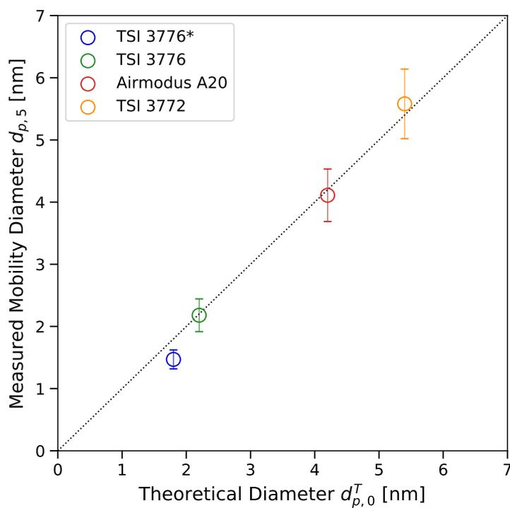
**Figure 7.** Theoretical Diameters: The Figure shows the theoretically minimal diameters necessary for particle activation of neutral silver seeds as a function of the measured 5 % cut-off diameter for negatively charged silver seeds. Every color corresponds to a different particle counter. Data points on the dashed line stand for the equality of the theoretical and measured diameters.
