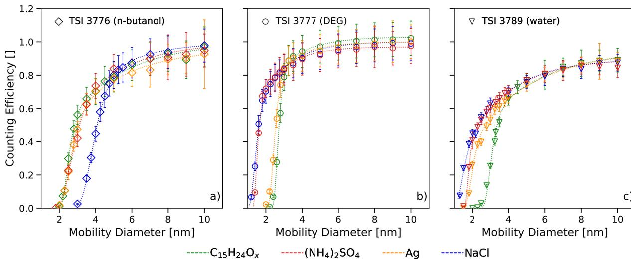
**Figure 2.** Detection Efficiencies and Working Fluids: The Figure shows the detection efficiencies for different seed particle materials as a function of the electrical mobility equivalent diameter. Different colors correspond to different seed particles and every plot is related to a different working fluid: n-butanol (Panel a), DEG (Panel b) and water (Panel c).
