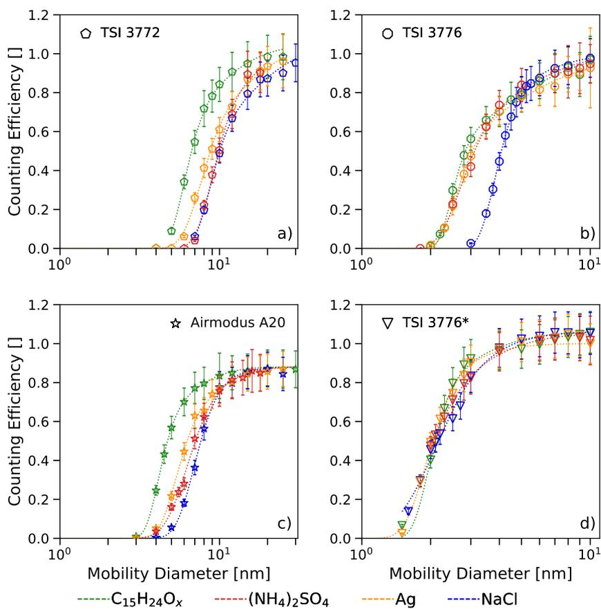
**Figure 4.** Detection Efficiencies of the Butanol-Based CPCs: The Figure shows the detection efficiencies as a function of the electrical mobility equivalent diameter. Every plot corresponds to a different butanol-based CPC: TSI 3772 (Panel a), TSI 3776 (Panel b), Airmodus A20 (Panel c) and TSI 3776\* (Panel d). The abscissa is scaled logarithmically to set focus on the dependence of the detection efficiencies on the seed particle material.
