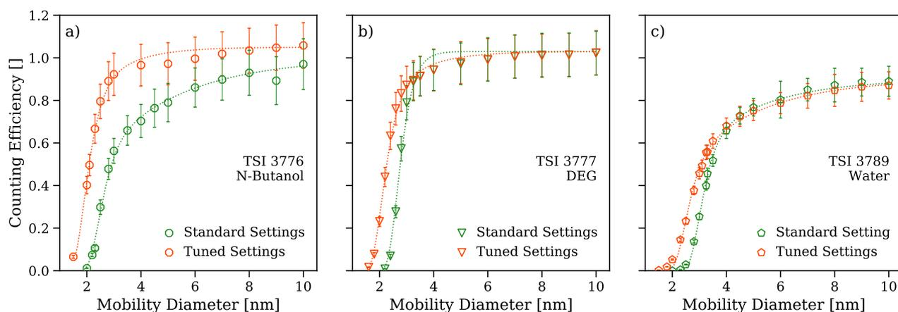
**Figure 6.** Detection Efficiencies of the Tuned Instruments: The Figure shows the detection efficiencies for BCYO<sub>x</sub> seeds as a function of the electrical mobility equivalent diameter. The green lines correspond to the standard settings, the orange ones to the tuned settings. Every plot shows data of a different instrument: TSI 3776 (Panel a), TSI 3777 (Panel b) and TSI 3789 (Panel c).
