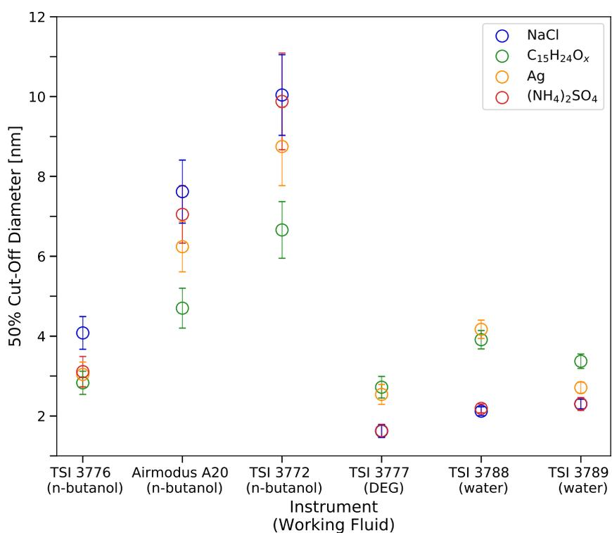
**Figure 5.** 50 % Cut-off Diameters for Different Working Fluids: The Figure shows the 50 % cut-off diameters measured with the TSI 3776, the Airmodus A20, the TSI 3772, the TSI 3777, the TSI 3788 and the TSI 3789. Different colors corresponds to different seed particle compositions.
