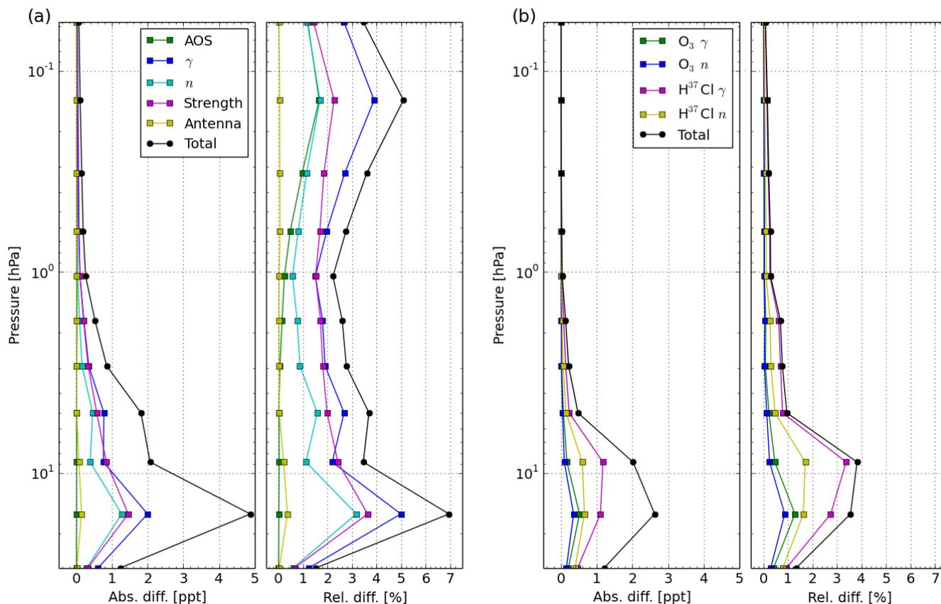
**Figure 4.** (a) Summary of absolute and relative differences derived from systematic errors of  $\text{CH}_3\text{CN}$  retrieval caused by uncertainties in the spectral parameters and (b) instrumental functions derived from single scan spectrum observed on November 4th 2009, in the Tropics, as shown in Fig. 3. The black line in the middle panel indicates the total error calculated by root-sum-square of all assumed error sources.
