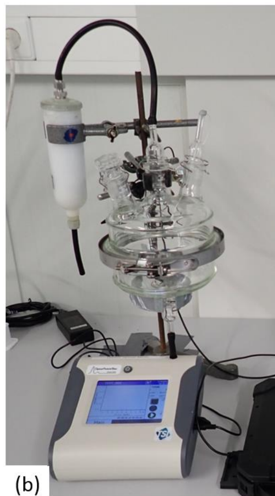
Figure 4: Setup used for laboratory experiments. The samples are placed in a glass cuvette in a vertical air stream. Air is supplied via an inlet with a filter connected to it; the outlet is connected to an OPS for particle measurements. A humidity and temperature sensor is placed inside the cuvette through an opening in the upper lid, which is sealed to avoid contamination. (a) Schematic drawing, and (b) close-up photograph.
