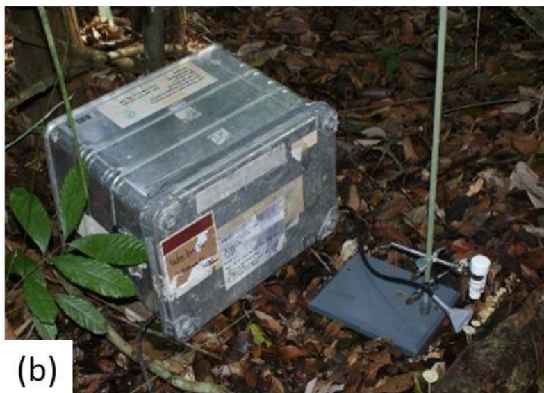
Figure 3: Setup used for field measurements. The optical particle sensor (OPS) is located in a box for weather protection. From this, an inlet ending with a funnel leads to the organism of interest. The setup is accompanied by a T/RH-sensor located in the direct vicinity of the sample (a) Schematic drawing, (b) overview photograph, and (c) close-up photograph of the described setup.
