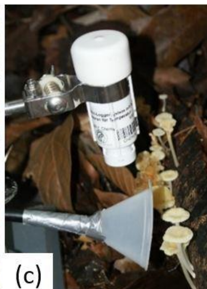
Figure 3: Setup used for field measurements. The optical particle sensor (OPS) is located in a box for weather protection. From this, an inlet ending with a funnel leads to the organism of interest. The setup is accompanied by a T/RH-sensor located in the direct vicinity of the sample (a) Schematic drawing, (b) overview photograph, and (c) close-up photograph of the described setup.
