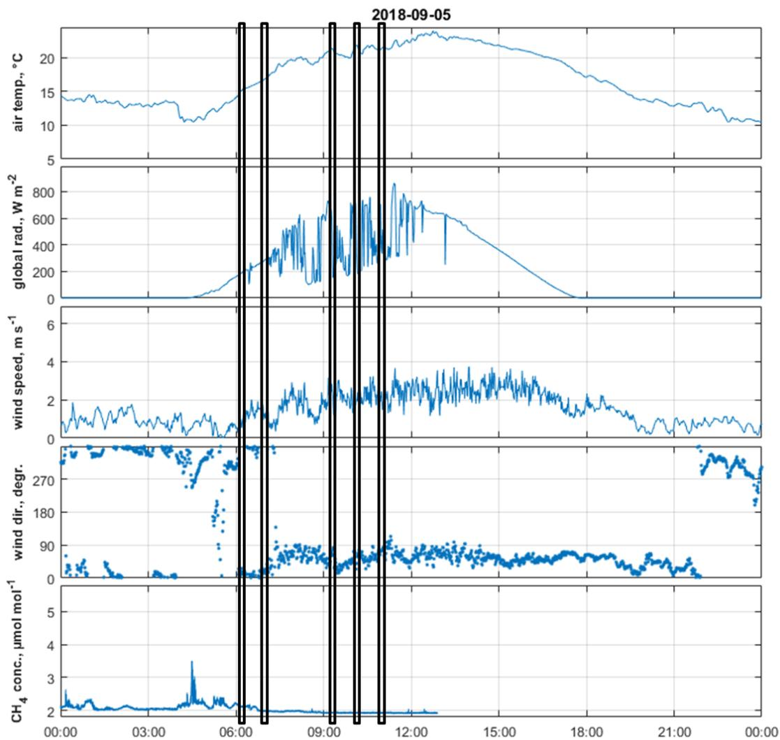
**Figure 4.** Diurnal course of the main meteorological parameters air temperature, global radiation, wind speed, wind direction, and methane concentration recorded at the meteorological mast at Zarnekow on 05 September 2018.
