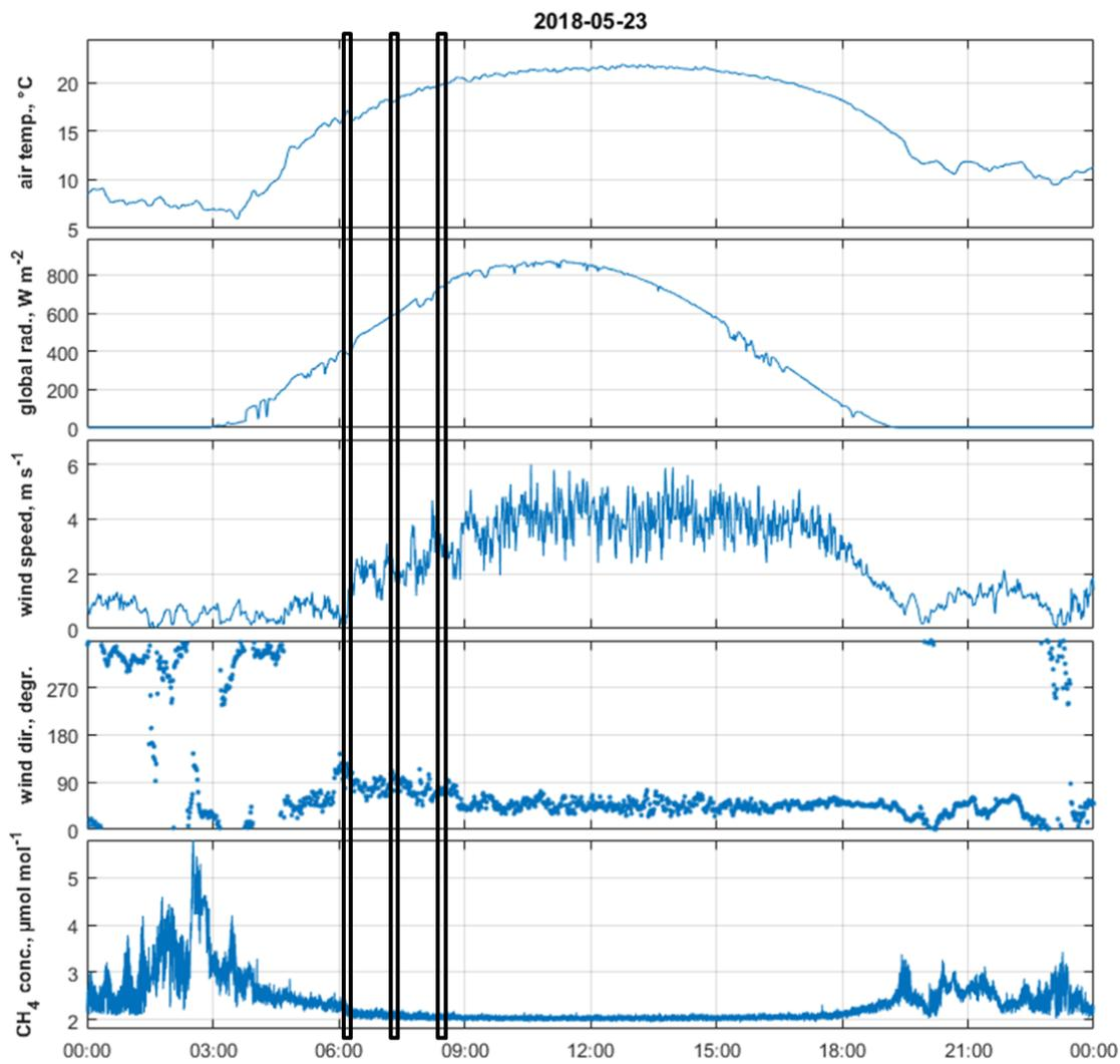
**Figure 3.** Diurnal course of the main meteorological parameters air temperature, global radiation, wind speed, wind direction, and methane concentration recorded at the meteorological mast at Zarnekow on 23 May 2018.
