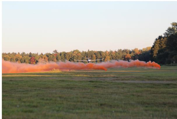
**Figure 5.** Illustration of concentration during stable stratification. The photo was taken at the air field Aue/Hattorf, Germany, on 2 October 2011 at 16:15 UTC, copyright Institute of Flight Guidance, TU Braunschweig
