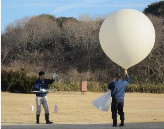
10 **Figure S1: Preparations for a flight launch at 8:30 local time on January 6, 2017. RS-11G and RS92 units were hung on the ends of a plastic/cardboard rod.**
