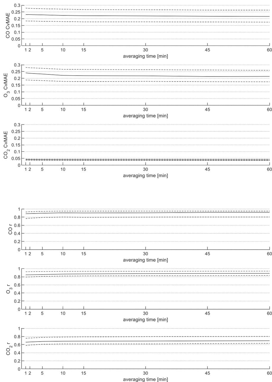
5 **Figure S5.** An evaluation of the performance of the calibration algorithms as a function of the averaging period; in contrast to the previous figure, this presents the results when averaging is performed after calibration, rather than before. In terms of CvMAE, performance improves as averaging time increases. In terms of Pearson r, results can be worse with longer averaging, due to the
