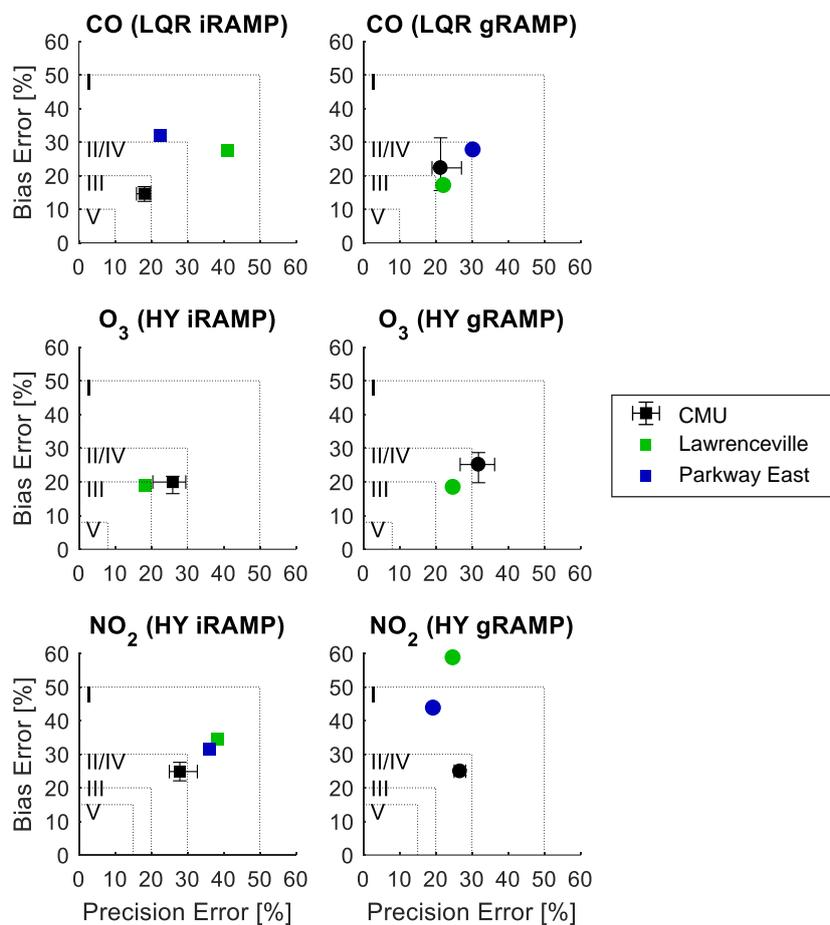
5 **Figure 5. Comparative performance of individual and general models for RAMPs deployed to ACHD monitoring stations using EPA performance criteria. Dotted lines indicate the outer limits of each performance tier. Performance shown for the CMU site is based on performance across all RAMPs at that site based on testing data only. Proximity to the lower-left corner of each figure indicates better performance.**
