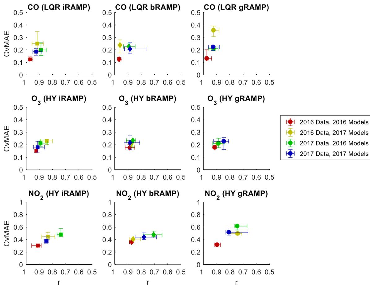
**Figure 6. Comparative performance of models in 2016 and 2017. The “Models” year indicates the year from which training data collected at the CMU site are used to calibrate the model; the “Data” year indicates the year from which testing data collected at the CMU site are used to evaluate the model.**
