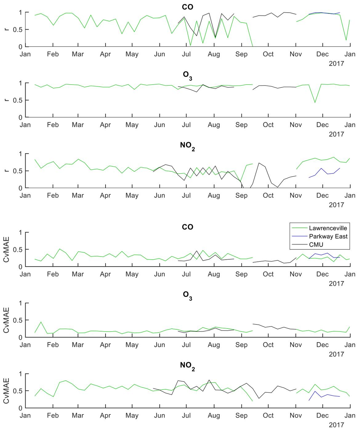
**Figure 7. Tracking the performance of RAMP monitors deployed to ACHD Lawrenceville, ACHD Parkway East, and CMU over time. Statistics are computed for each week. Results shown correspond to those of models trained using data collected at the CMU**
