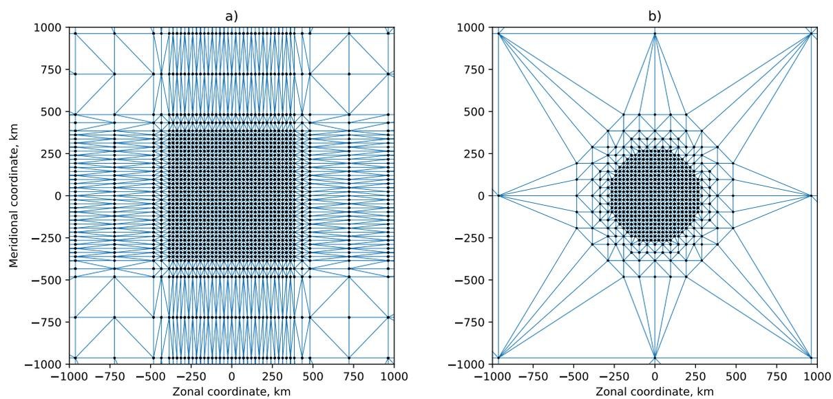
**Figure 1.** Horizontal cuts of retrieval grids. Dots show grid points, blue lines indicate Delaunay cell boundaries. Panel (a) shows the full initial grid for retrievals A, B, C (all horizontal layers of this grid are identical), panel (b) shows the thinned out grid for retrieval D (cut at 11 km).
