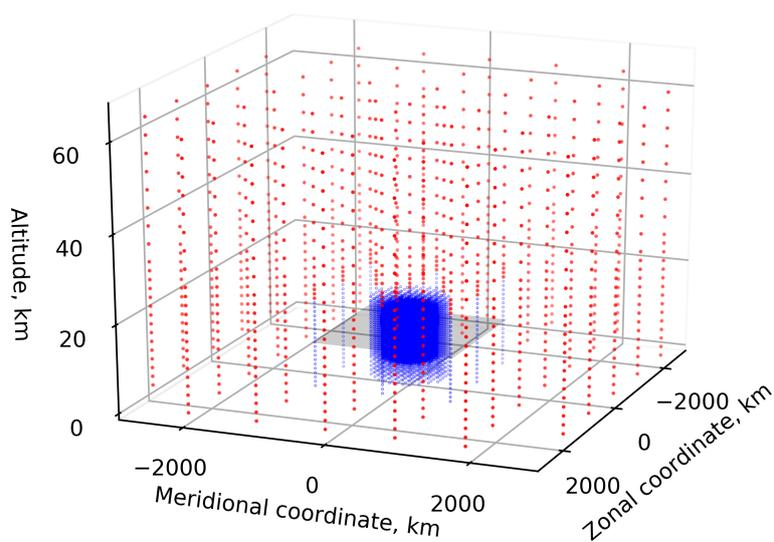
**Figure 2.** Grid for retrieval D. Radial distance is defined as distance to the vertical line at the centre of the hexagonal flight path ( $66^{\circ}\text{N}$ ,  $15^{\circ}\text{W}$ ). Points within the inner core ( $1000\text{ km} \times 1000\text{ km} \times 20\text{ km}$ ) are shown in blue, other points – in red, shaded rectangle shows the position of horizontal cut in Figure 1b.
