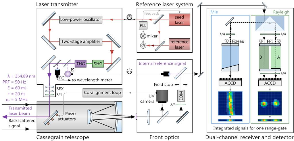
**Figure 1.** Schematic of the ALADIN Airborne Demonstrator (A2D) wind lidar instrument consisting of an injection-seeded, frequency-tripled laser transmitter, a Cassegrain telescope, front optics and a dual-channel receiver. PLL: phase locked loop, SHG: second harmonic generator, THG: third harmonic generator, IS: integrating sphere, FC: fiber coupler, BEX: beam expander, EOM: electro-optic modulator, FPI: Fabry-Pérot interferometer, ACCD: accumulation charge-coupled device.
