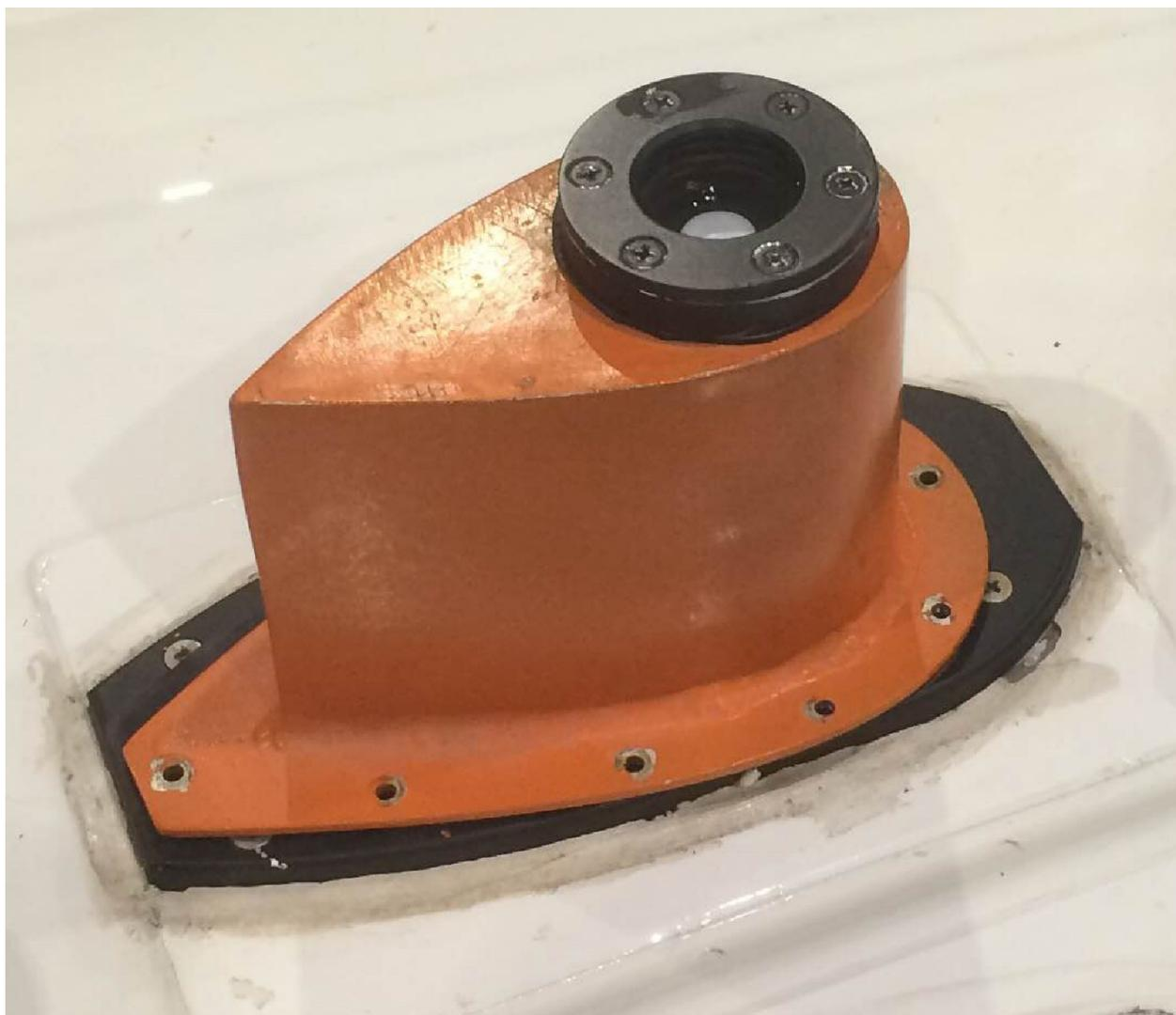
**Figure 1.** The zenith mounted OrangeCan on top of the NASA LaRC UC-12B aircraft. The RCR optic was mounted inside directly under a BK7 optical window to characterize sky conditions during flight.
