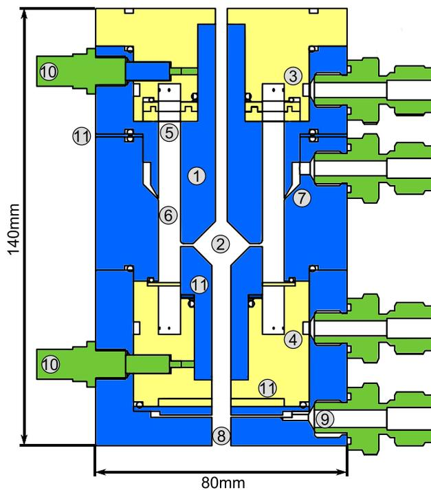
**Figure 2:** Schematic quarter section of the DMA unit of the TD-DMA with 1) central electrode, 2) collection area, 3) sheath flow inlet, 4) sheath flow outlet, 5) tissue for laminarising the sheath flow, 6) selection area, 7) aerosol inlet, 8) outlet for the filament, 9) aerosol outlet, 10) SHV supplies and 11) spacer plates. Conductive stainless steel parts are shown in blue, isolating PEEK parts in yellow.
