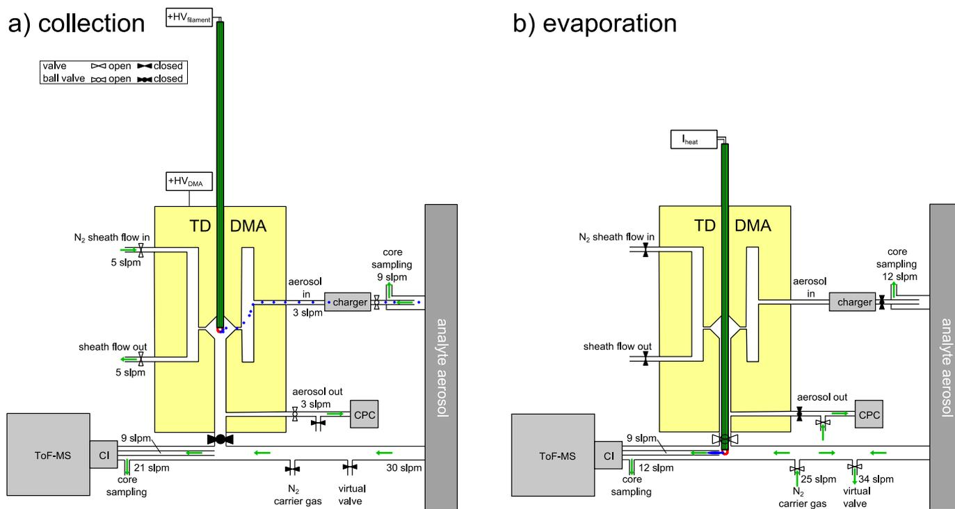
**Figure 1:** Measurement setup of the TD-DMA with step a) collection, and b) evaporation. Filled valves correspond to closed, unfilled ones to open. In step a, particles (blue) from the aerosol sample are charged, size selected and collected on a filament (red) inside the DMA-unit (yellow). In step b, the filament is moved in front of a mass spectrometer and the collected material is evaporated and analyzed.
