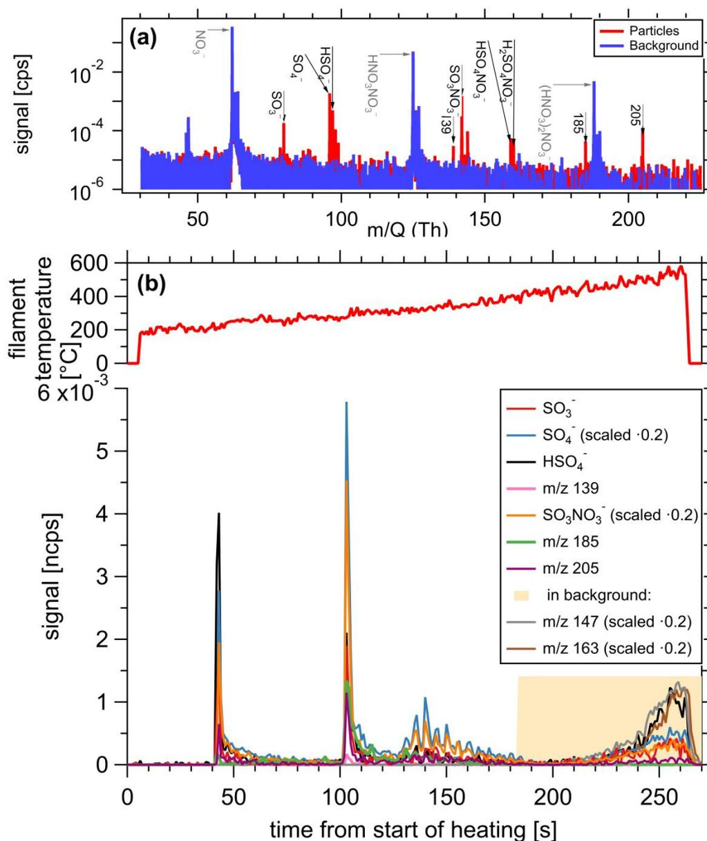
**Figure 8:** Composition measurement of 15 nm particles generated from dimethylamine, sulfur dioxide and ozone in presence of UV light. a) Spectrum of particle phase compared to the background. Prominent particle phase peaks in black, primary ions in grey. b) Time series of evaporation. With increasing filament temperature, substances desorb from the filament and are depleted rapidly. At high temperatures, signals originating from the inlet line appear.
