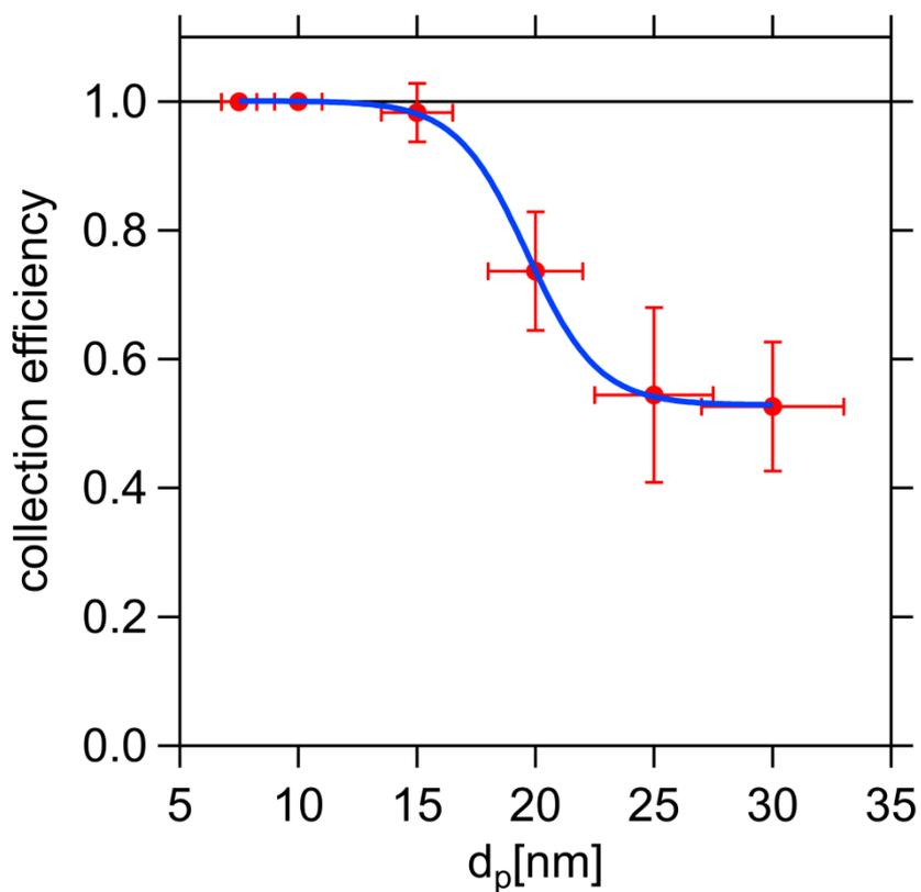
**Figure 6:** Collection efficiency depending on the particle size. Due to the decreased electrical mobility, the required collection voltage increases with particle size, which currently limits the collection efficiency at larger sizes.
