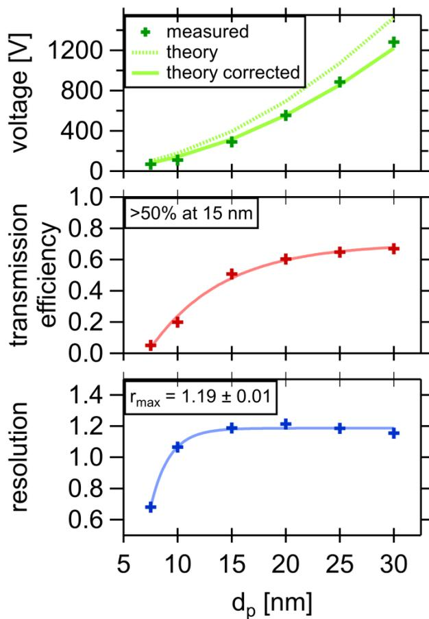
**Figure 5:** Summary of DMA performance parameters. The DMA is optimized for a coarse resolution and high transmission in order to collect a maximum amount of particle mass while still allowing size selection.
