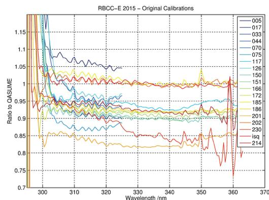
**Figure 2.** Average ratios to QASUME calculated from all UV data measured during the Huelva 2015 comparison campaign. The calibrations were provided by the operators of the instruments. Figure from Gröbner (2015).
