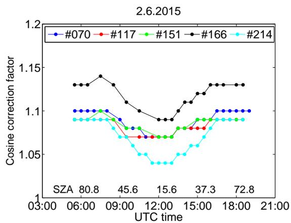
**Figure 5.** Diurnal variation of the cosine error correction factor of Brewers #070, #117, #151, #166 and #214 at 308 nm on 2nd June 2015. The X-axis is time (UTC), but SZAs are shown for 6, 9, 12, 15 and 18 UTC.
