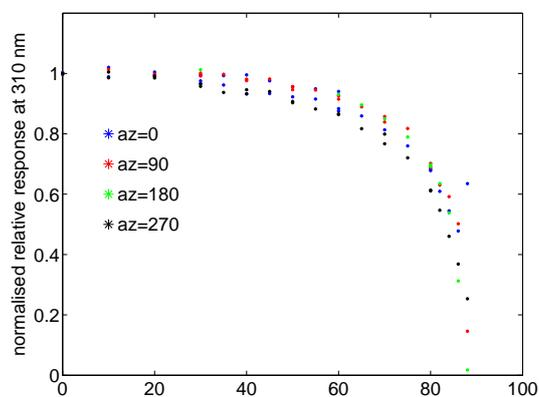
**Figure 3.** The cosine error of Brewer #214, FMI, Sodankylä, measured during the QASUME site audit in 2014. Results are normalized to the ideal cosine response.
