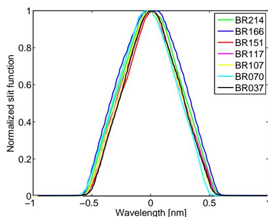
**Figure 1.** Slit functions of Brewers no. 037, 070, 107, 117, 151, 166 and 214. The results are normalized to the maximum and the x-axis is wavelength (nm) relative to the peak center.
