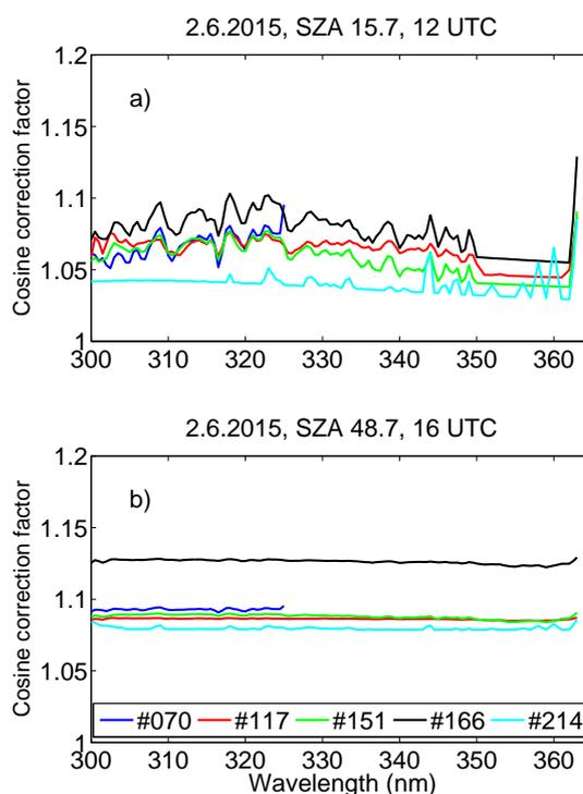
**Figure 6.** Spectral variation of the cosine error correction factor of Brewers #070 #117 #151 #166 #214 during one UV scan at a) 12 UTC (SZA 16°) b) 16 UTC (SZA 49°) on 2nd June 2015.
