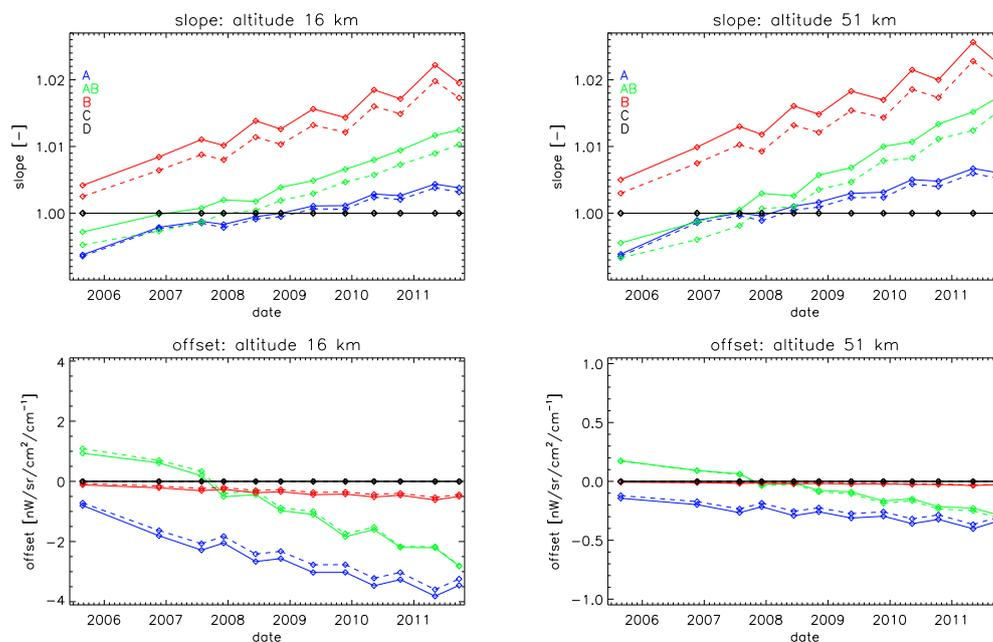
**Figure 5.** Slope and offset of the linear fit of MIPAS RR Level 1 Spectra with the old set of NL coefficient versus spectra with new set of NL coefficients at 16 km (left) and 51 km (right). Solid lines correspond to forward mirror movement, and dashed lines correspond to reverse mirror movement.
