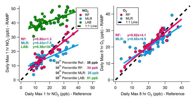
Figure 12: Performance of one representative RAMP (RAMP#1) for NAAQS compliance metrics (O<sub>3</sub>: Daily Max 8 h, NO<sub>2</sub>: 98<sup>th</sup> percentile of Daily Max 1 h averages) Right: comparison of daily 8 hr maximum reference monitor ozone concentrations (x-axis) to MLR and RF models. Left: comparison of daily 1 h maximum reference monitor concentrations versus the LAB, MLR and RF models. The NO<sub>2</sub> standard is the 98<sup>th</sup> percentile of the daily 1 h maximums.
