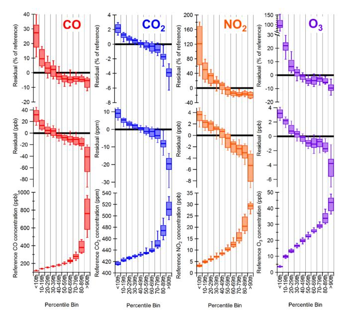
Figure 10: Box plots from the 19 RAMP monitors of median concentrations measured by monitors (bottom) and median model residuals (middle) and model residuals normalized to the reference concentration (top) for each pollutant, divided into deciles. The box plots provide the range of medians by the different RAMP monitors.
