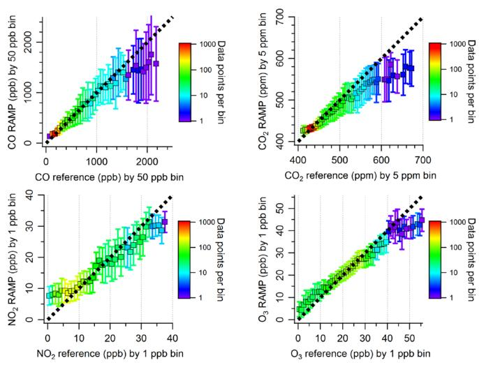
Figure 11: Illustrating the range of predictions from the 500 trees for RAMP #1. The testing data were binned and averaged. The concentration measured by the reference monitors is then plotted against the average concentration from the model. The error bars represent the standard deviation of the answers from the 500 trees and the bins are colour coded by the number of data points within each bin. The dashed black line is the 1:1 line.
