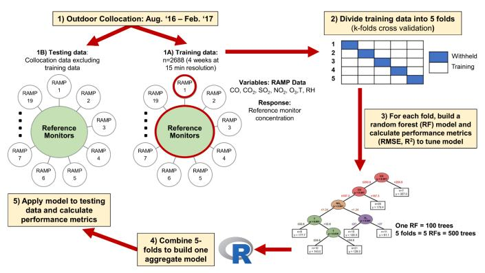
Figure 3: Flow path for data collection and RF model fitting and testing. From collocation period, 2688 points were sub-selected as training (1A) data while the remaining data were used for model testing (1B). The training data were further divided into 5 cross-validation folds and each fold was used to tune and build an RF model. All five models were then combined in R to build one cumulative model and the predictive power of the model was assessed for the withheld testing data.
