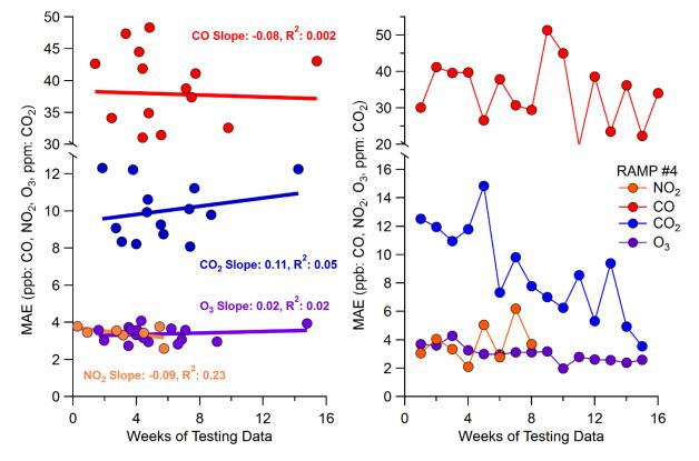
Figure 8: *Left:* Mean absolute error (MAE) versus the length of the testing period for CO (red), CO<sub>2</sub> (blue), NO<sub>2</sub> (orange) and O<sub>3</sub> (purple) for all the RAMPs. *Right:* Changes in MAE over time for the RAMP with the longest testing window (RAMP #4). The figure shows that the MAE is generally unchanged (or in some cases improves) as the amount of testing data increases, suggesting the RF models are stable over long periods.
