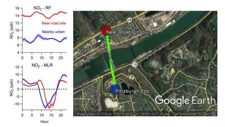
Figure 13: Left: Diurnal NO<sub>2</sub> patterns at two nearby sites (one urban, one near-road) measured by RAMP monitors calibrated using RF models (top) or MLR models (bottom), Right: Satellite view of the two sites, which were ~1.5 km apart. The urban site was at the Pittsburgh Zoo and the near-road site was within 15 m of Highway 28.
