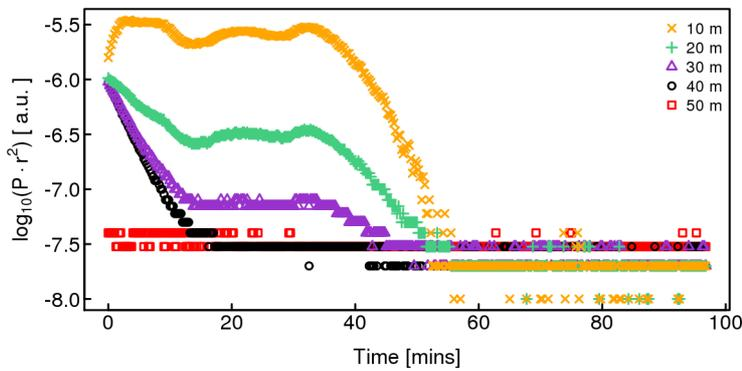
Fig. 4: ~~Manufacturer~~: Logarithm of range-corrected signal reported  $RCS = P \cdot r^2$  in the first five range gates during a termination hood measurement of LUMO sensor A with firmware 1.72.
