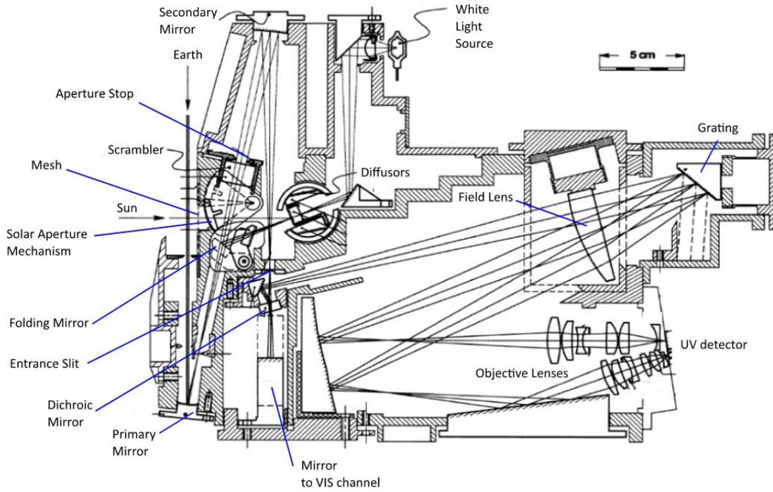
**Figure 2: Optical design of the UV channel. The telescope (Primary and Secondary mirror) is used for both channels. The visible light that passes the dichroic mirror is coupled into the VIS channel. The Folding Mirror is depicted in two positions (earth view and sun / calibration view).**
