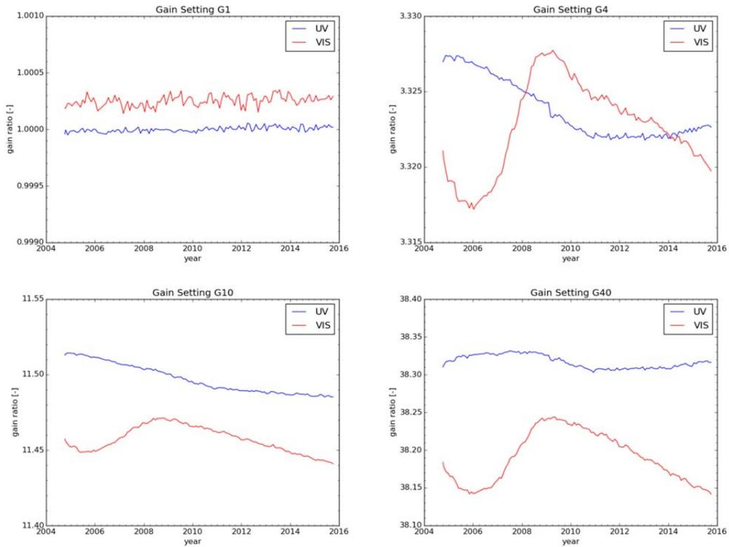
**Figure 8: Gain ratios trends over the mission time for the four gain settings. The very small deviation from 1 for gain setting G1 in the VIS channel (upper left panel) is an indication of the accuracy of the analysis method.**
