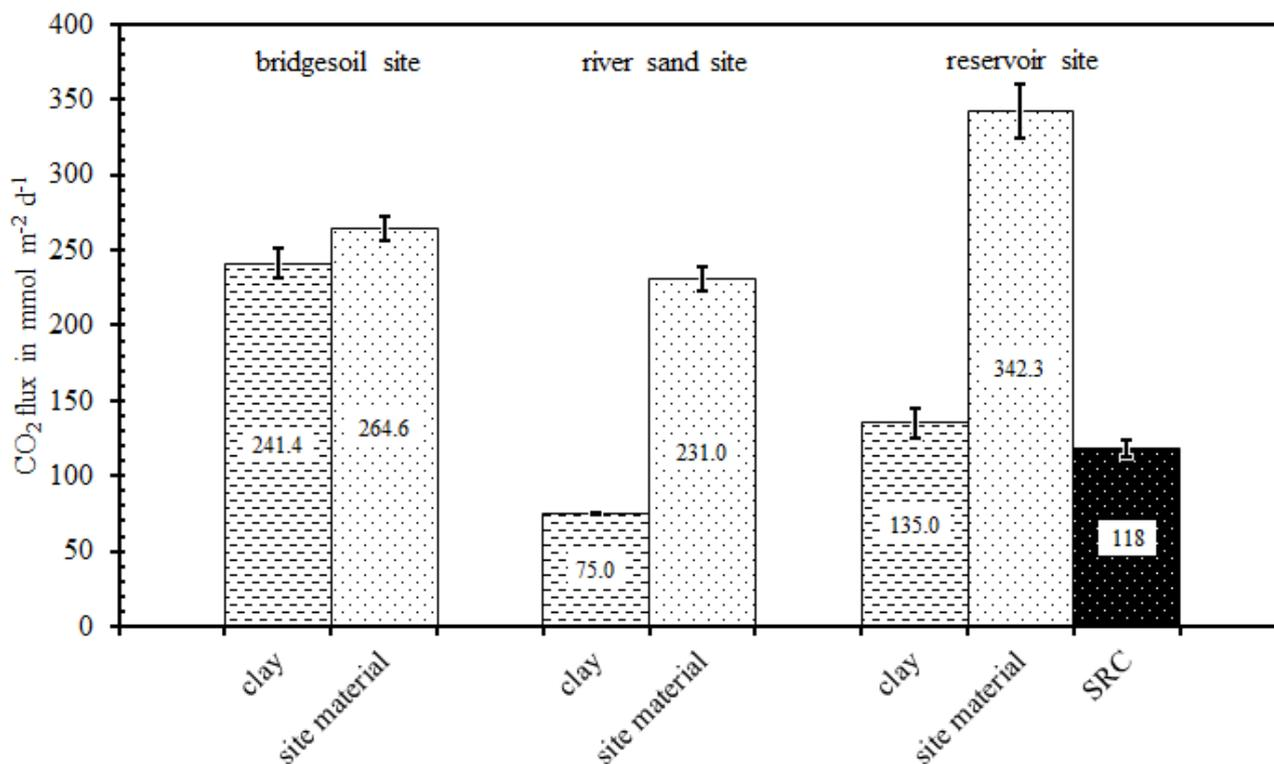
Figure 2: Mean CO<sub>2</sub> fluxes detected in the different sample groups during field experiments (mean ± SD, n = 3; reservoir site n = 4). SRC = soil respiration chamber + IR analyser, sealed with clay.
