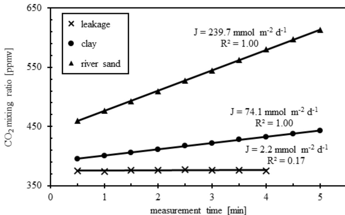
Figure 3: Example showing typical progression of CO<sub>2</sub> concentration during field measurements with clay and ambient material (example: river sand site).
