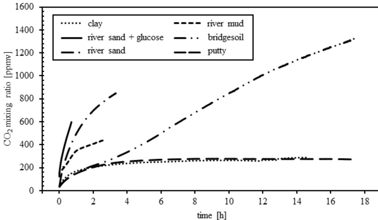
**Figure 1: CO<sub>2</sub> concentration during long-term laboratory chamber experiments with different sealing materials.**
