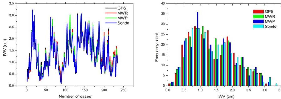
**Figure 2.** Example of the time series (left) of integrated water vapor obtained with the instruments available at the Lindenberg site (reported in Table 1) and histograms (right) of the frequency count of the time series shown in the left panel. After detrending of the time series, the histograms were used to calculate entropy and mutual correlation.
