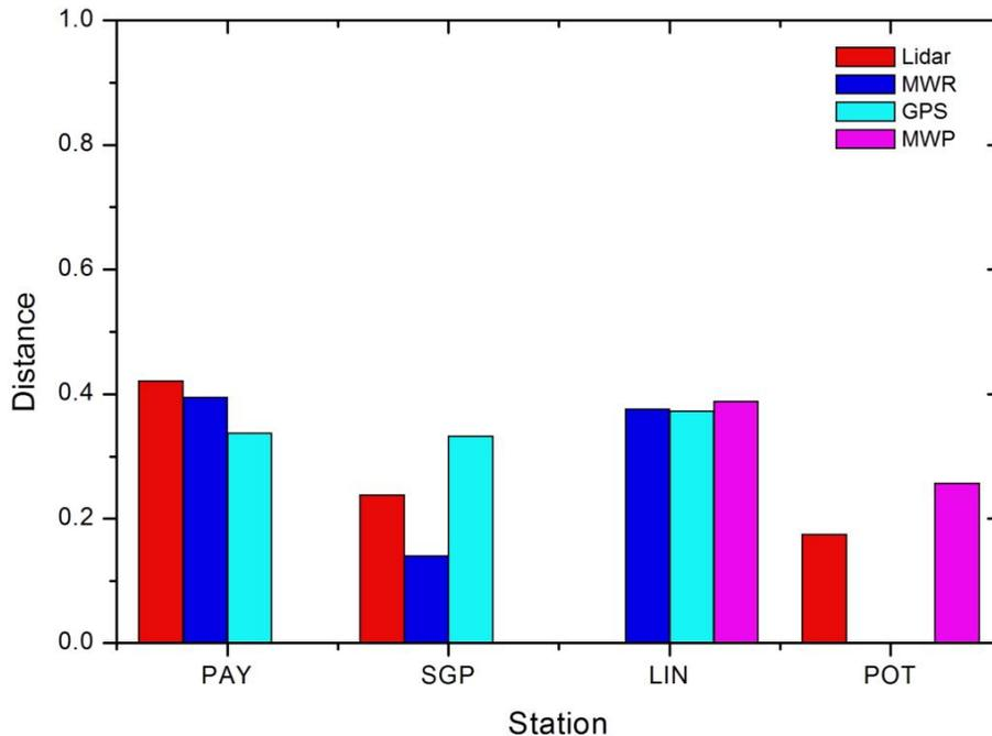
**Figure 4.** Comparison of the statistical distances between pairs of times series data retrieved for the instruments measuring integrated water vapor with respect to the time series obtained from the radiosondes at the Payerne (PAY), Southern Great Plains (SGP), Lindenberg (LIN) and Potenza (POT) sites.. The data set considered includes all available measurements in 2010–2012.
