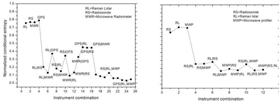
**Figure 7.** Comparison of the normalized conditional entropy values retrieved for all combinations of instruments measuring integrated water vapor at the Southern Great Plains site (left panel) and the Potenza site (right panel).
