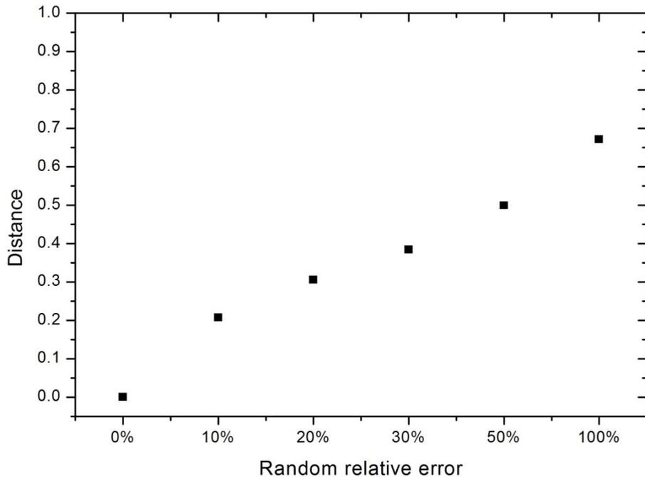
**Figure 9.** Statistical distance between the integrated water vapor time series retrieved from the radiosonde at the Lindenberg site and the corresponding time series obtained by adding random noise to the radiosonde time series to simulate the effect of increasing relative random uncertainty.
