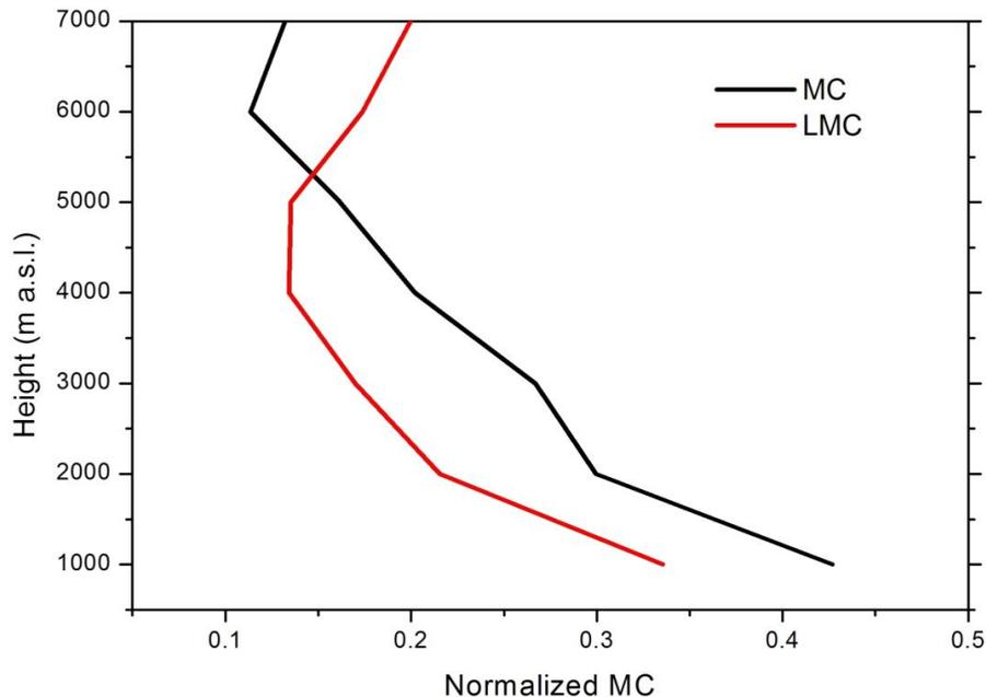
**Figure 8.** Comparison of the normalized mutual correlation for the Linear (LMC) and Non-Linear Cases (MC), calculated for the lidar and radiosonde data sets from the Potenza site.
