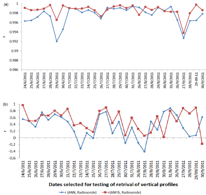
Fig. 4. Pearson product movement correlation coefficient ( r ) between radiosonde temperature (a) and humidity (b) profiles and retrieved profiles using ANN and ANFIS.
