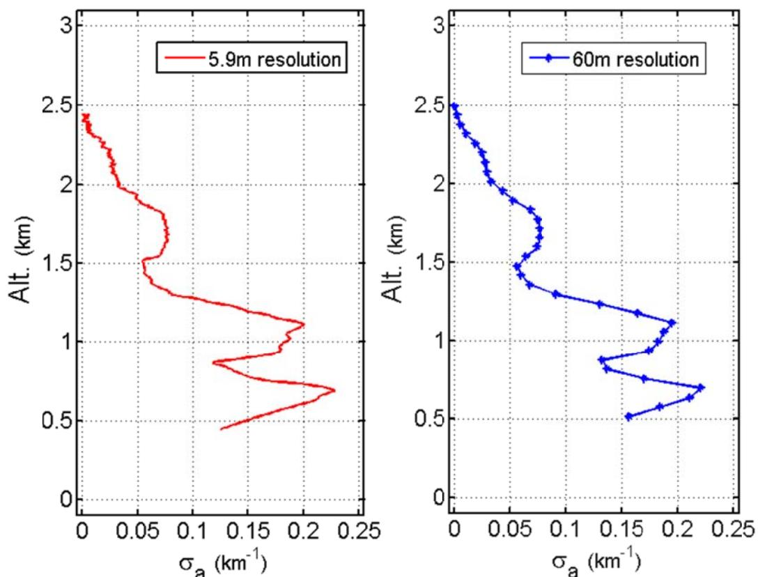
We can see that although we lose small details in the profile, the main structures are not meaningfully affected by the change in the resolution.
