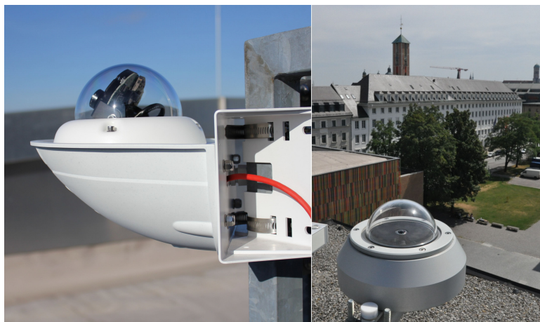
Fig. 1. Wide-angle camera in Oberpfaffenhofen (OP, left panel) and Munich (MIM, right panel). The sphere in the top-cross of the St. Markus church, above the MIM camera, is used as southeastern landmark.
