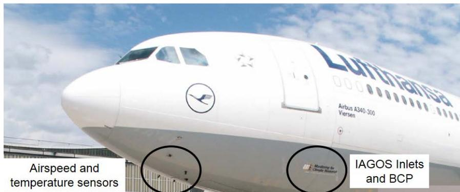
**Fig. 13.** The BCP is shown here mounted on the Lufthansa Veirsen A340-300 Airbus, as part of the IAGOS instrument package. Also shown are the locations of the aircraft airspeed and temperature sensors.
