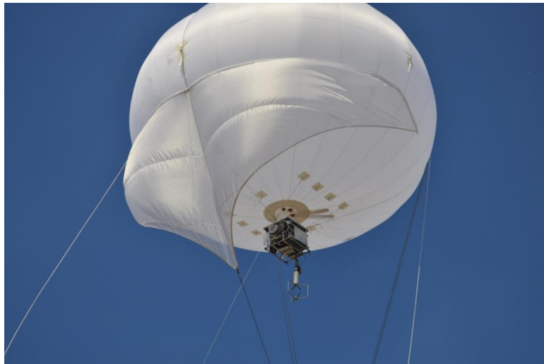
Fig. 1. Photograph of Aerostat based sampling system equipped with the 3-D anemometer mounted below the samplers.
