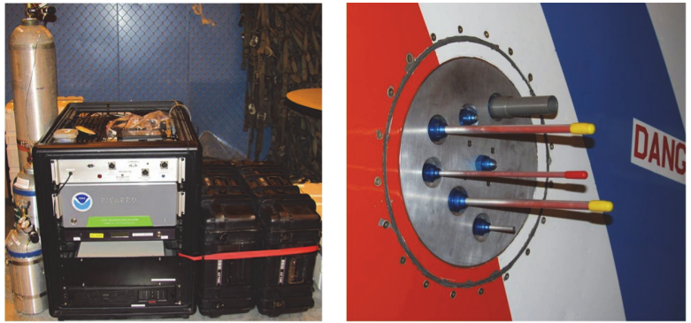
Fig. 2. NOAA equipment pallet for USCG C-130: three reference gas cylinders, instrument rack, and two Programmable Flask Packages (PFPs) (left). Window replacement inlet plate (external view) (right).
