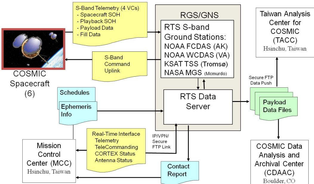
**Fig. 4.** FS-3/C Ground System Data Flow.
