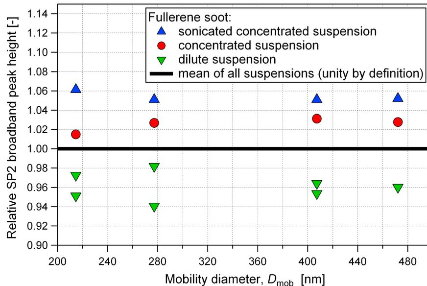
**Fig. 5.** Effect of different fullerene soot suspension treatments on the SP2 calibration based on particle selection by a DMA. The relative SP2 broadband peak height is obtained by division of the broadband peak height measured for a certain suspension by the mean value of the broadband peak heights measured for all suspensions at equal mobility diameter.
