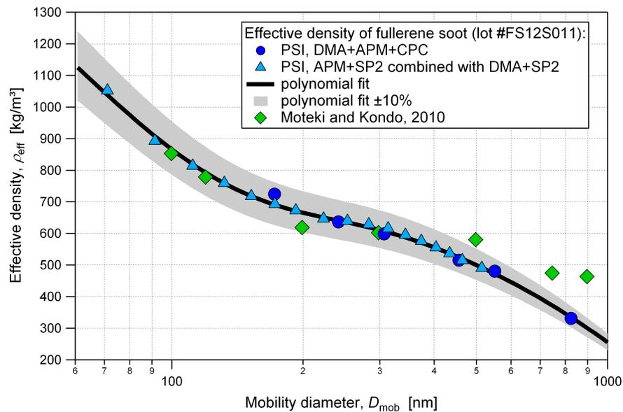
**Fig. 4.** Effective density of fullerene soot as a function of mobility diameter.
