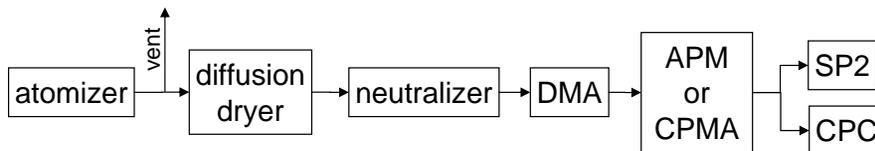
**Fig. 1.** Experimental setup for effective density measurements.
