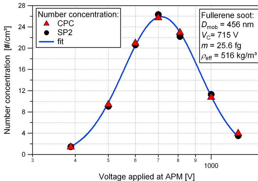
**Fig. 2.** Classification of fullerene soot particles with mobility diameter  $D_{\text{mob}} = 456 \text{ nm}$  with the DMA-APM system (APM operated at 2000 rpm).
